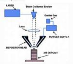
The figure below shows a simple control setup of the AM system. In this research, we only focus on the temperature control.
